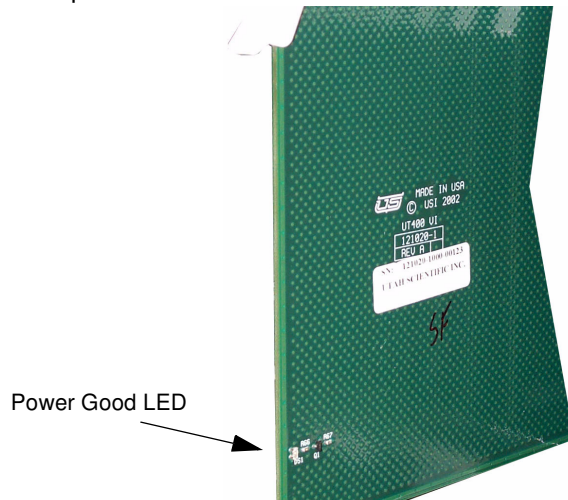
FIGURE 2-4. Power Good LED
